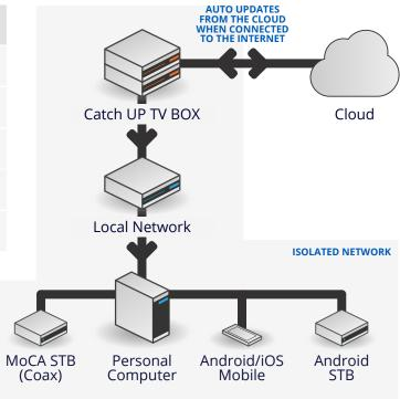
The TikiLIVE local delivery platform has been designed to accommodate remote installations who have limited Internet delivery options. This plug-n-play solution allows you to deliver and service multi dwelling or closed communities via a multi-casting or uni-casting network.
